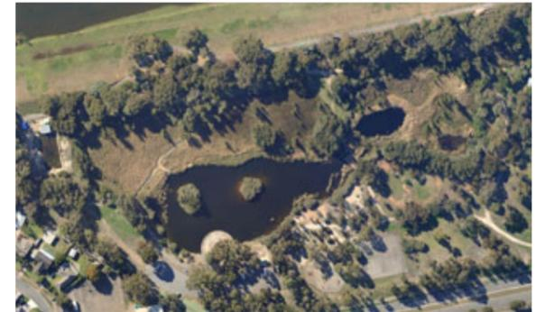
The wetland was built in 1993 to detain and improve stormwater prior to discharge into the River Torrens, which then flows into Gulf St Vincent. Stormwater pipes divert water into the wetland which consists of 2 ponds that filter water through reed beds. The larger pond retains water all year round, while the smaller pond holds additional stormwater flow during winter. When stormwater input exceeds the ponds' capacity water overflows into an adjoining pump station.
