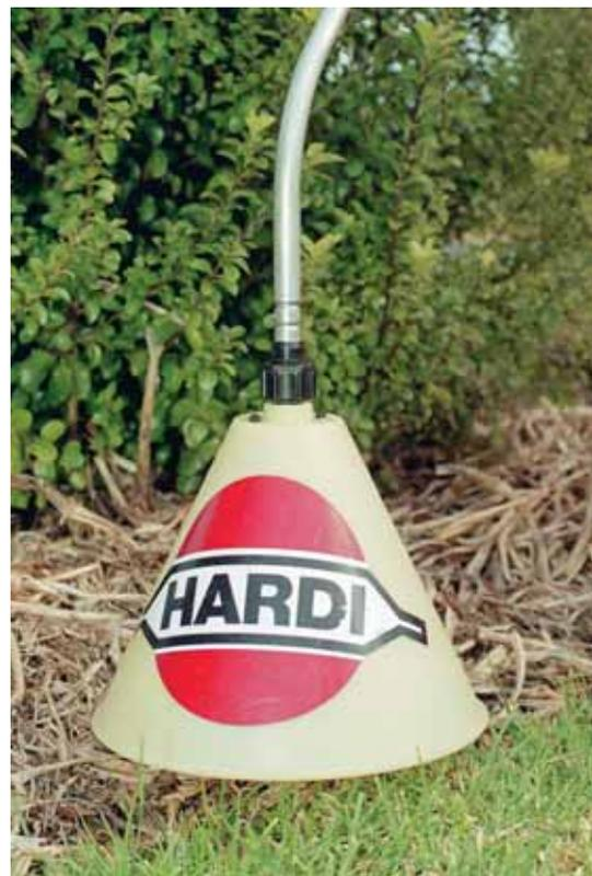
*If using a cone nozzle, it should be shrouded to ensure the spray doesn't go off-target*
