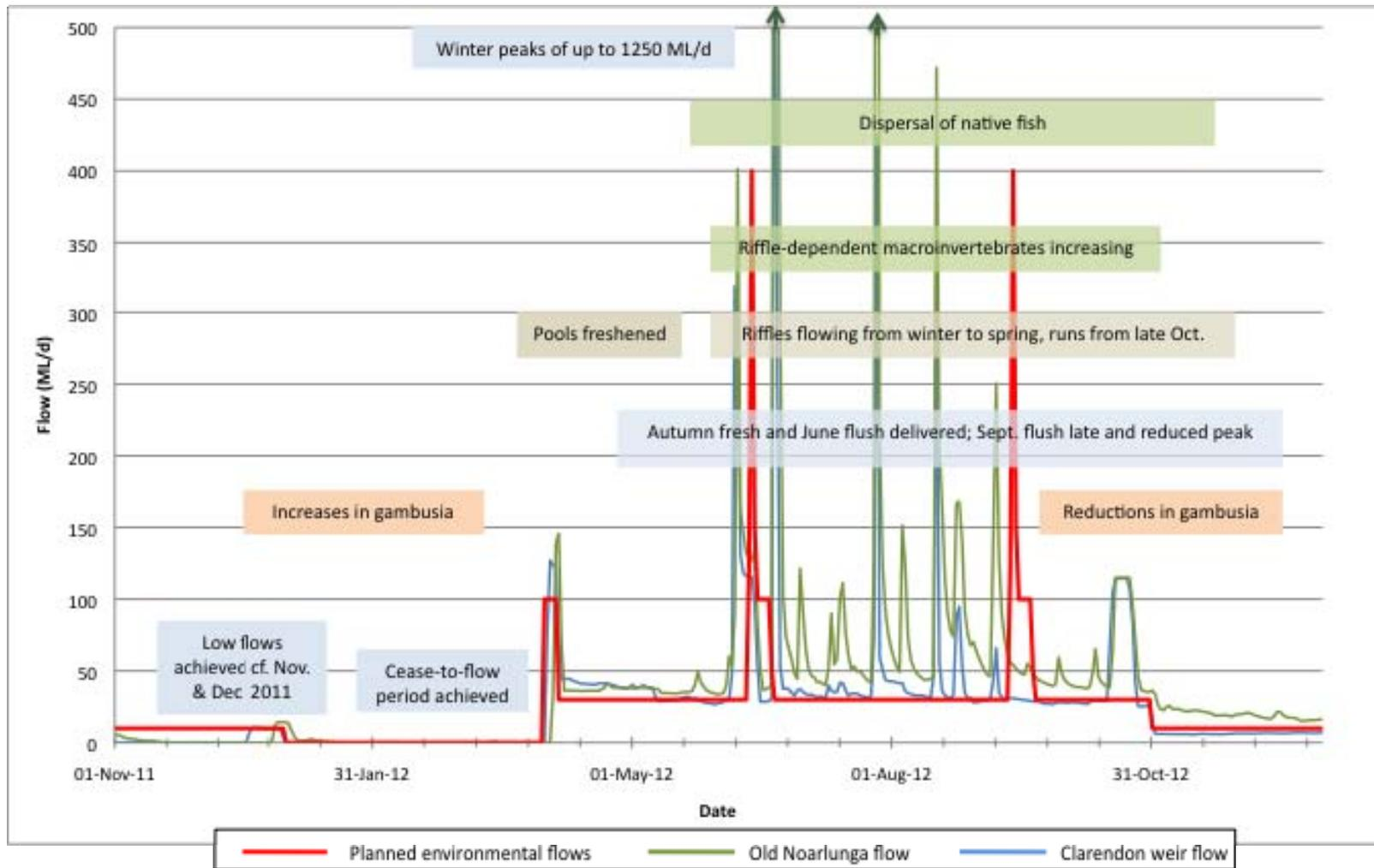
Figure 9: Onkaparinga River trial reach hydrology, as measured downstream of the Clarendon Weir and downstream at Old Noarlunga, showing key flow events and environmental outcomes for Year 1, November 2011 to December 2012
