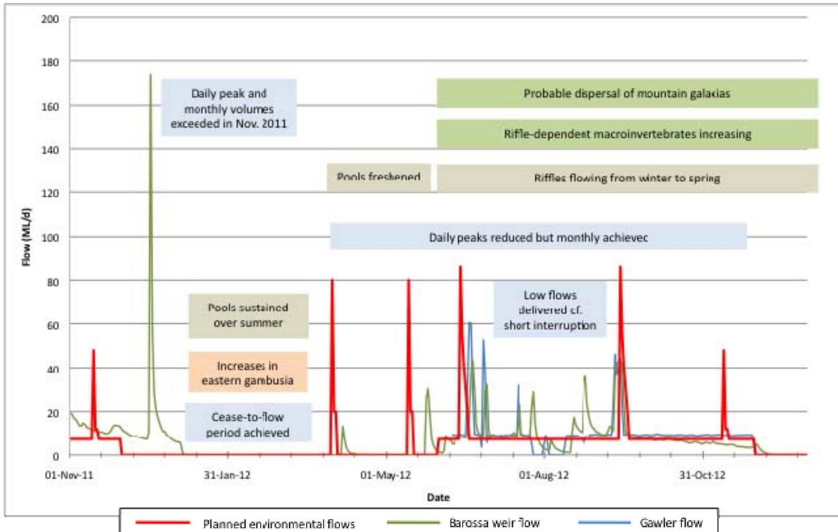
Figure 8: South Para River trial reach hydrology, as measured at the weir and upstream of Gawler, showing key flow events and environmental outcomes for Year 1, November 2011 to December 2012
