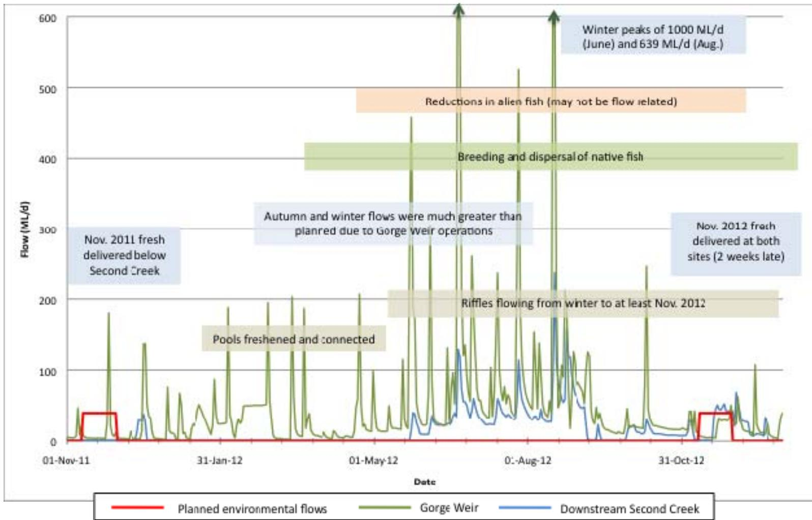
Figure 11: River Torrens – Gorge Weir to Torrens Lake trial reach hydrology, as measured at the weir and below the Second Creek junction, showing key flow events and environmental outcomes for Year 1, November 2011 to December 2012
