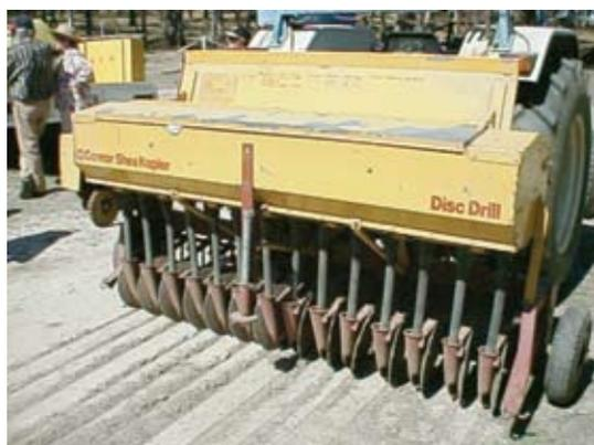
Figure 9: Seeding machine with disc drill suitable for re-seeding pastures
