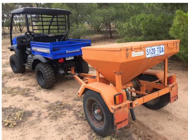
Figure 2. Bait laying machine for towing behind a vehicle
