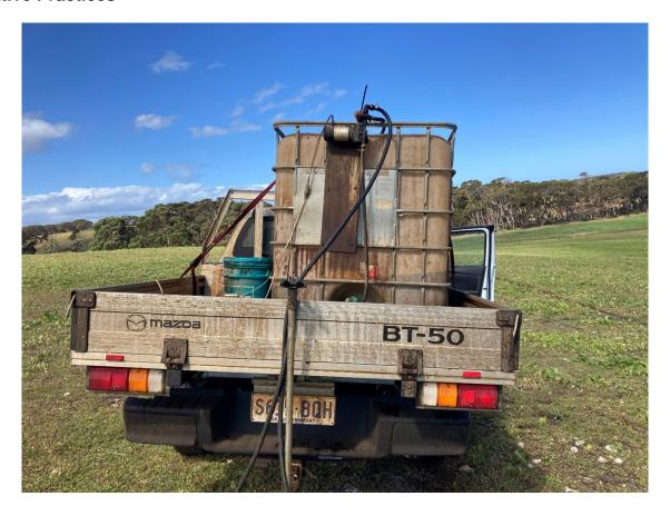
Tim made the stand for a spray unit for the KILB that can be connected to a tow ball. This is used to spray out bio stimulants and biological treatments such as EM and compost and vermicaste extracts made on farm. If only there was a more efficient way to clean the car afterwards!
