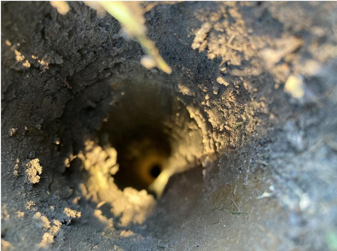
This photo shows the 3 metre hole that is left after the soil core was removed for analysis. Because the elevation of the property and its proximity to the ocean, the testing allowed us to look for sea water.
