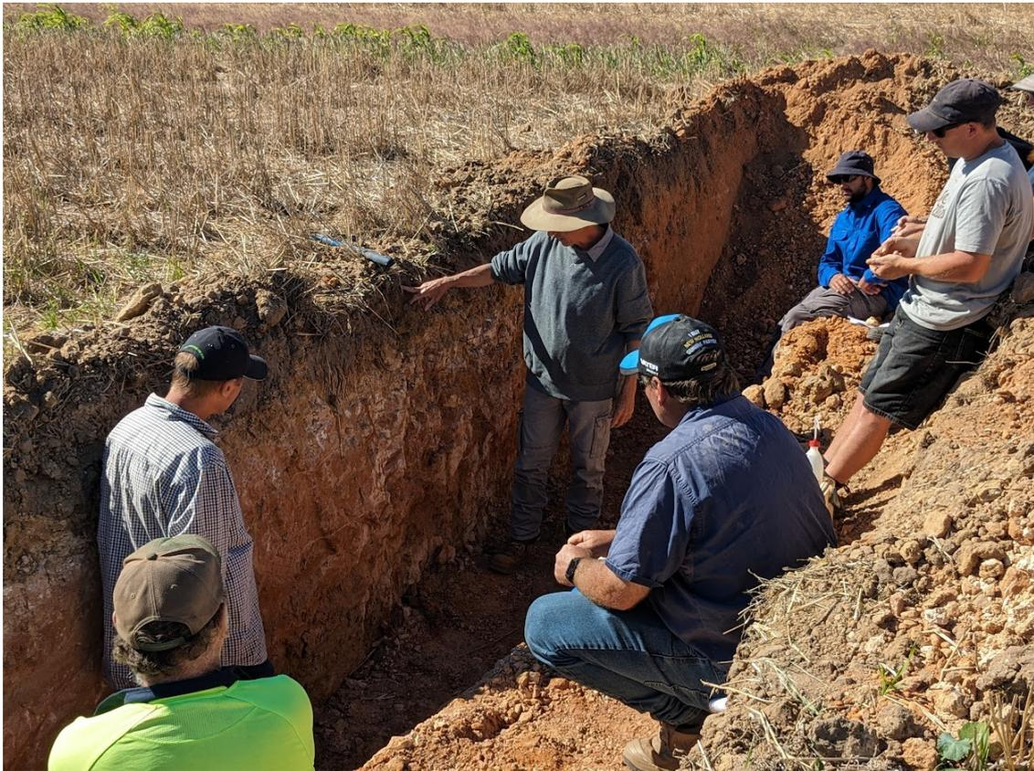
While the soil pit is available and the horizon levels are visible, soil samples can be taken for laboratory testing:
